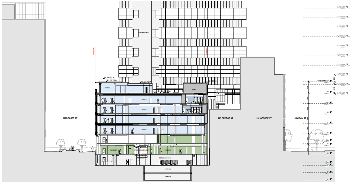
Figure 23: Proposed north-south section through the George Street podium
